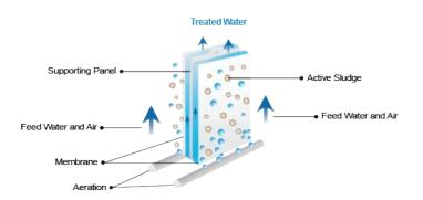
MBR combines conventional activated sludge technology with membrane filtration. MBR can be designed at a much higher mixed liquor suspended solids (MLSS) concetration compared to conventional processes, giving advantages of lower hydraulic retention time (HRT) and higher sludge retention time (SRT). This reduces the footprint of the overall wastewater treatement.
