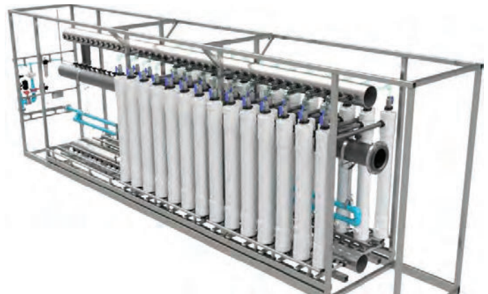
Figure 2: 3D CAD model of UF rack after the retrofit showing additional room for installation. Image courtesy of WesTech Engineering, Inc.
