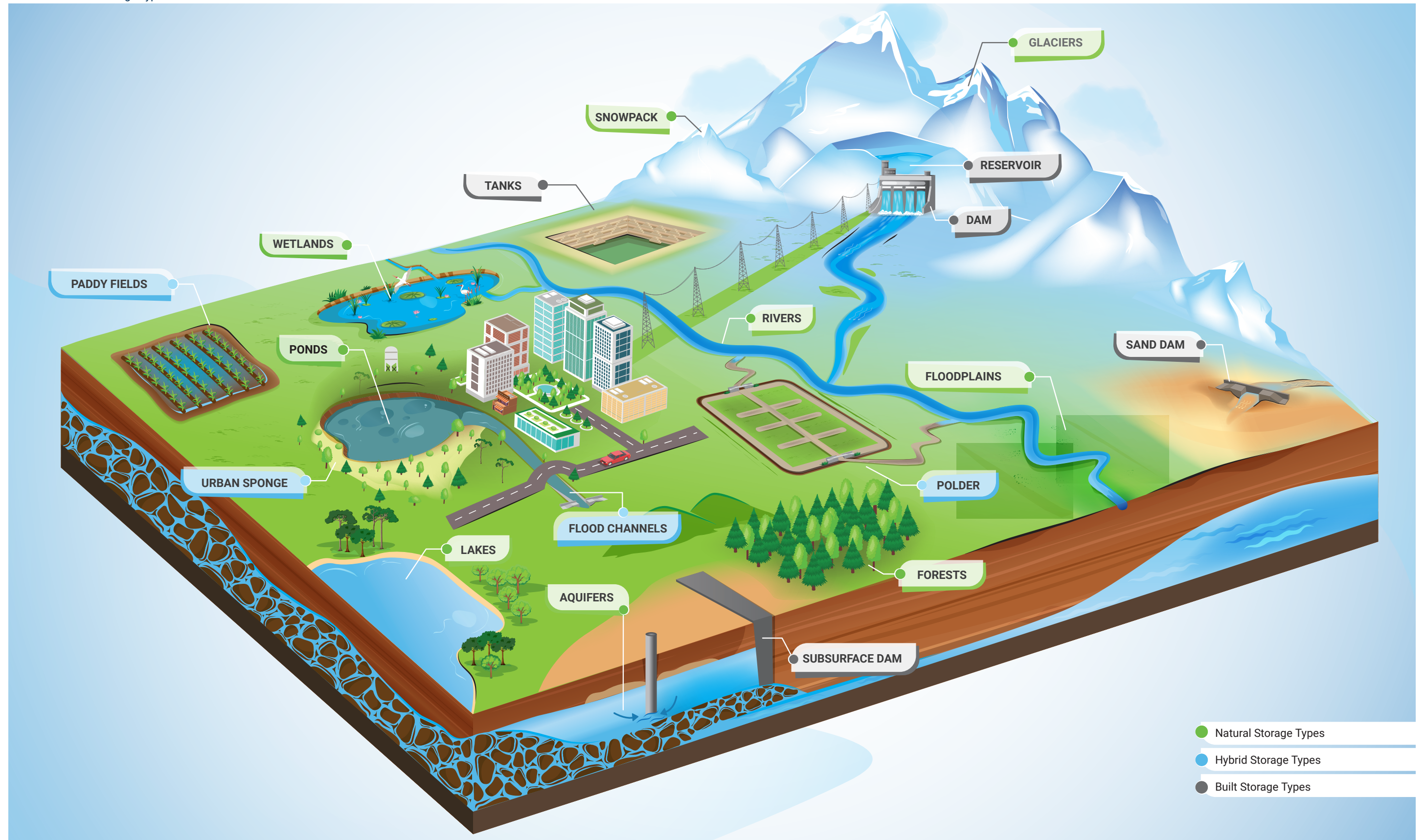
FIGURE 2.1 Water Storage Types
