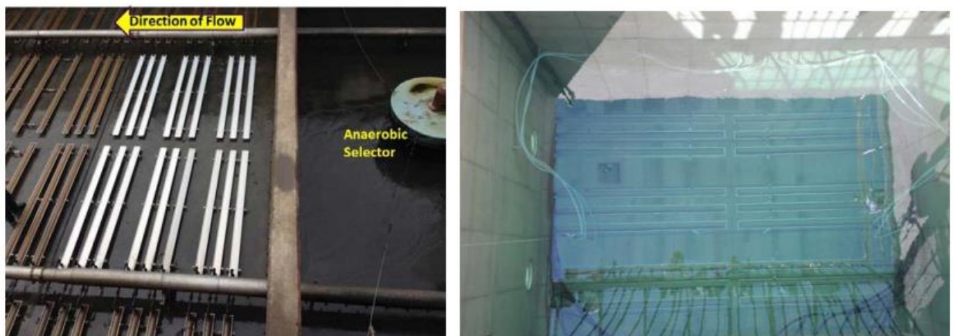
Figure 3. Left photo shows the location of the eighteen eleven-year old diffusers harvested for clean water and material strength testing (represented by replacement with the new diffusers). Right photo shows the harvested diffusers in the test tank for clean water testing
