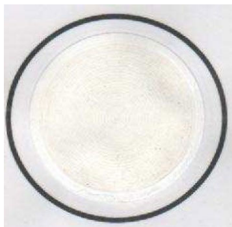
Figure 4 – Ultrafiltrated water SDI
