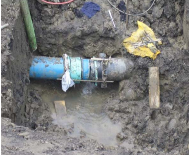
Figure 2.10 Restrained mechanical coupling leak at transition from HDPE to PVC
