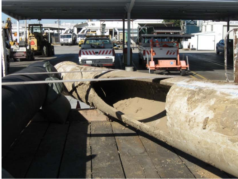
Figure 2.1 AWWA C900 PVC pipe failure in 2009 due to large pressure fluctuations
