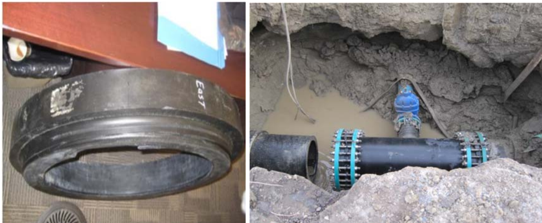
Figure 2.9 HDPE butt fusion joint failure in Edmonton, Canada
