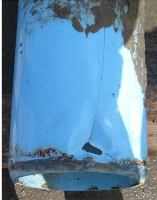
Figure 2.5 Erosion of pipe material from a poorly sealed joint
