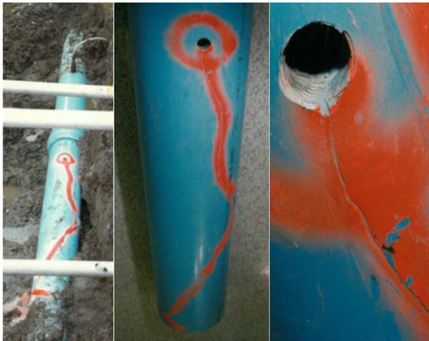
Figure 2.5 Erosion of pipe material from a poorly sealed joint
