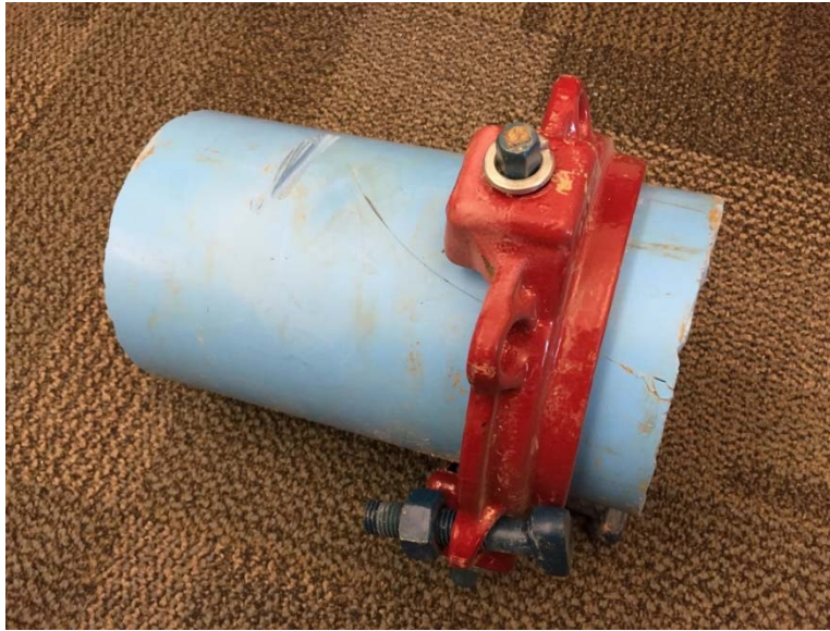
Figure 4.2 WaterOne PVC (C900) pipe failure
