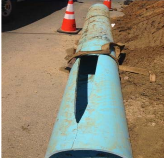
Figure 2.3 PVC pipe failure due to tapping at California American
