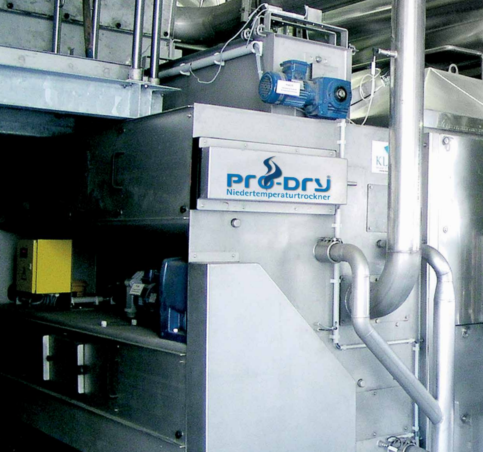
Pro-Dry® 2/1 (top), rotational heat exchanger (center), air channel system for heat recovery (right)
