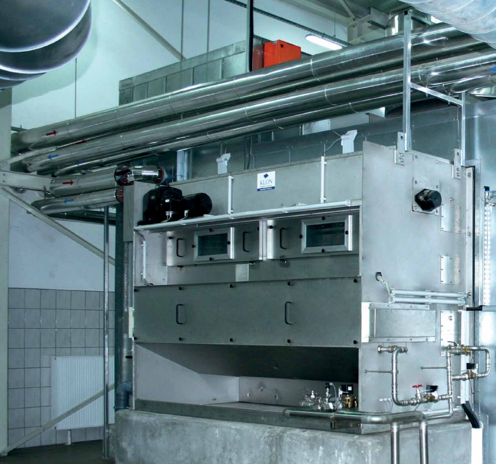
Pro-Dry® 2/2 (top), air fans (center), distributor (right)
