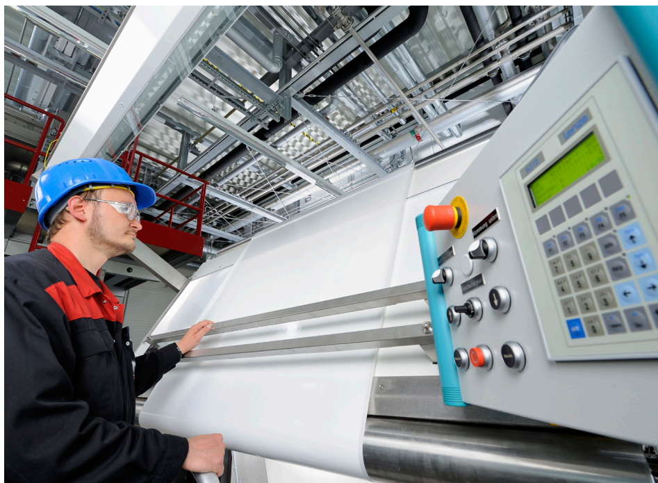
The membranes are based on a three-layer composite structure that is manufactured in several production stages.
